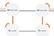
Radio Link Aggregation is a mechanism that doubles radio capacity aggregating two radio channels. The master unit splits incoming data traffic proportionally over the master and slave modulation schemes. The two radio channels can be either provided by XPIC or 2\*(1+0) systems.
