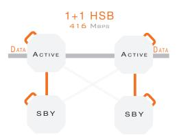
In 1+1 HSB, only the Active transmitting unit is switched on. Upon failure on this unit, the Stand-by takes over, switching on its own transmitter, enabling data to flow through the protection branch.
