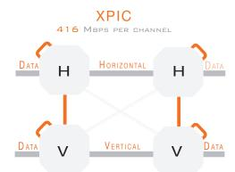
The XPIC system allows to double radio spectrum efficiency. Opposite polarized signals are cancelled out at receiver side. The two channels H and V are independent, reaching a maximum of 416 Mbps each. The best utilization of XPIC is in combination with the Radio Link Aggregation.
